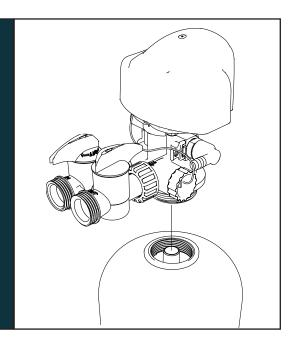
After media is added, remove the plug from the distributor tube, and fill the tank the rest of the way (up to the bottom of the tank threads) with water. This will allow the filter media to soak while the installation process is completed. Make sure that tank threads are clean and free of any media fines, and screw the control valve back onto the tank.
